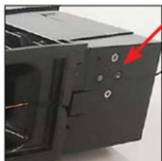
Push on the LED closest to the antenna on your Endura® Twist device to open the signal.
