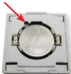
In order to reset the button control, one should activate the screen and push the reset button on the backside of the button control for > 5 seconds.
