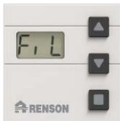
Whenever the filters need to be replaced, 'FiL' will appear on the display.
